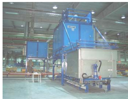
Motorised quench tank.
